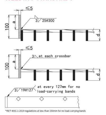
at each bearing bar for load-carring toe plates loading carrying
