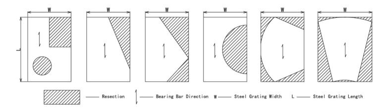
According to YB/T4001.1-2019, the area calculation principle is as following: The area of the steel grating is calculated based on the external rectangular area (WxL), without deducting the area of the cutout.
